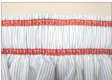
Making 2 line of flat lock stitch in one operation
